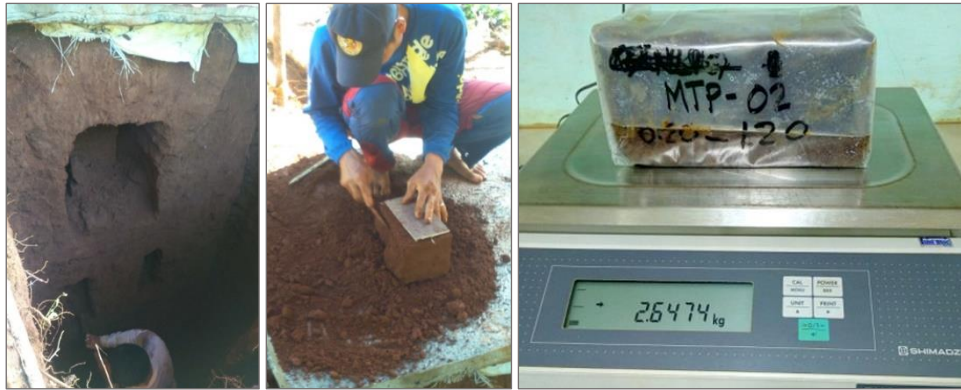
Figure 10-5. a) Samples were collected along the side of the test at 1 meter interval, b) sample was cut carefully to the desired dimension, c). sample sealed in plastic sample bag was weighed using digital scale at MMDC assay laboratory.
