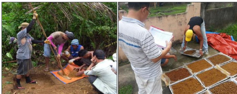
Figure 5-2. In-fill auger drilling and sample drying done by Xinbaoyuan as contracted by Asia Pilot.
