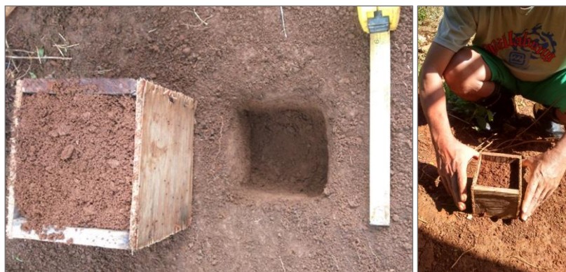
Figure 10-6. a) material was collected from a 10cm x 10cm hole and transferred to fabricated wooden box measuring 10cm x 10cm x 10cm until full, b) wooden box was lifted 10cm from the ground and dropped for compaction.
