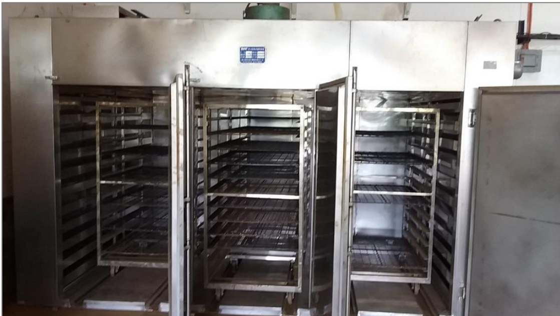
Figure 10-12. Electric oven for sample drying.
