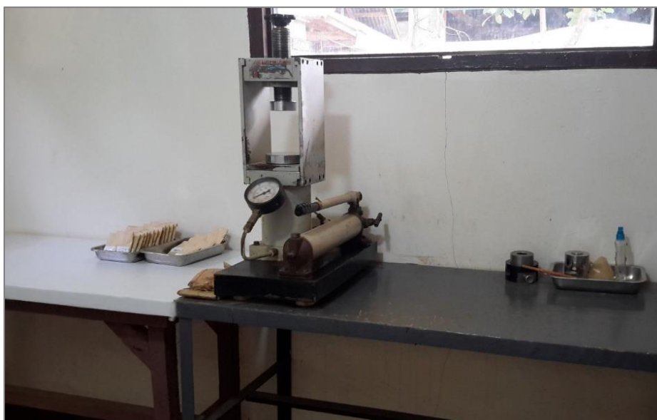
Figure 10-13. Hydraulic press for sample pelletizing.
