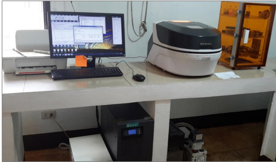
Figure 10-14. XRF-EDS Shimadzu brand with computer unit.
