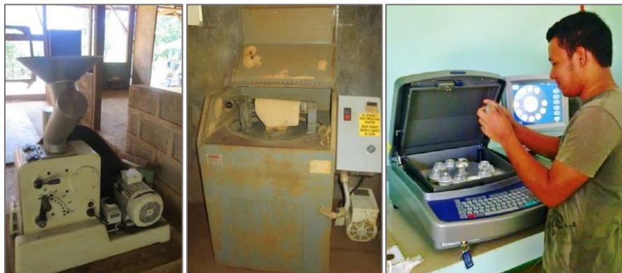
Figure 10-8. a) Crusher used for size reduction, b) pulverizer used to further reduce the size of the sample after splitting, c) X-Ray Fluorescence (XRF) Spectrometer at MMDC laboratory.
