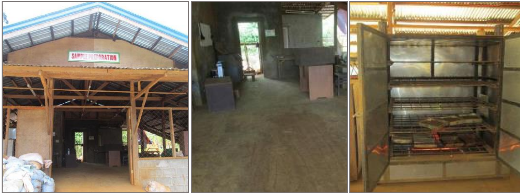
Figure 10-7. a) MMDC Sample Preparation Facility in Carrascal, Surigao del Sur, b) steel plates installed on the floor of the Sample Preparation Facility, c) electric oven used for drying samples.
