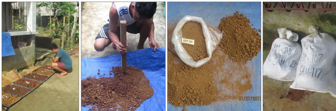
Figure 10-4. a) Sample sun drying, b) manual crushing of samples, c) coning and quartering, d) packing of samples in sacks.
