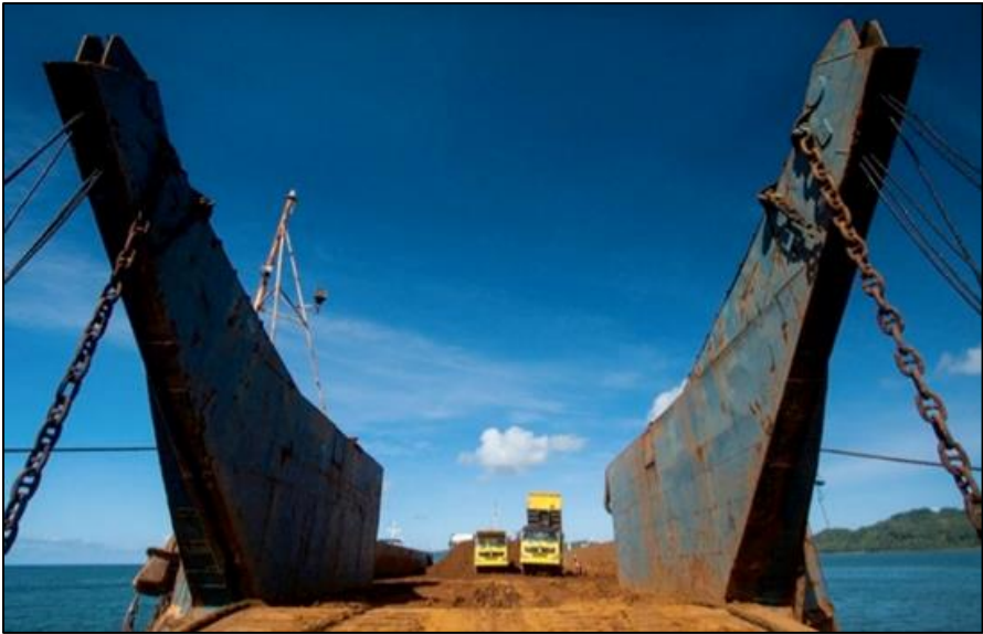
Figure 6-5. Loading of ore to LCT.
